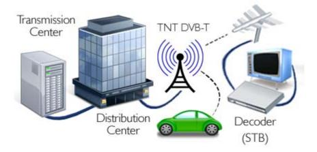
DTTV is transmitted on radio frequencies through the airwaves that are similar to standard analogue television. DTTV is received via a digital STB, or integrated receiving device (even portable), that decodes the signal received via a standard aerial. DTTV can also be received by computers equipped with a TV tuner card (component that allows television signals to be received by a computer).
